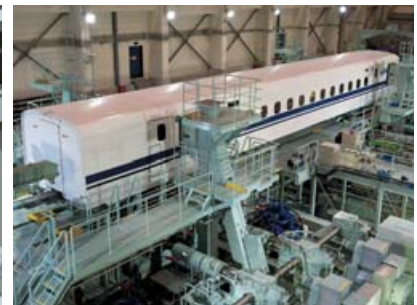
▲Rolling Stock Field Test Simulator
