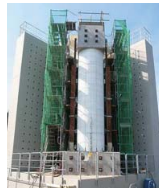
▲Tri-axial Loading System for Structures
